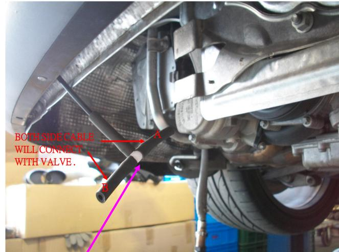
WHEN YOU PUT VALVETRONIC MUFFLER IN AND CONNECT WITH VACUUM TUBE (A \ B), YOU ARE REALLY COMPLETED INSTALLATION.
