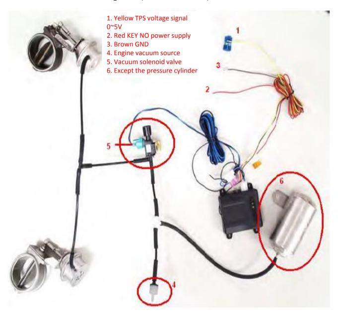
Second. Look for the power control box (KEY OIV POWER⊕), body grounding (GNDΘ) and throttle valve (TPS 0~5V signal).
