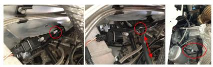
Place the cylinder as shown below: Loosen the screw and securely place the cylinder. Then tighten the screws and connect the silicone tube.
