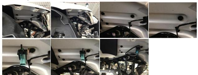
B. The Blue/Black solenoid wire is routed into the interior through the left rear wheel wall panel.
