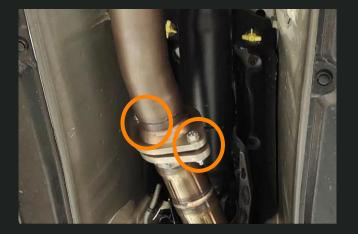
**Step 3**Install the Mid pipe-1 back onto the vehicle, then tighten the bolts connect it to the front pipe.
