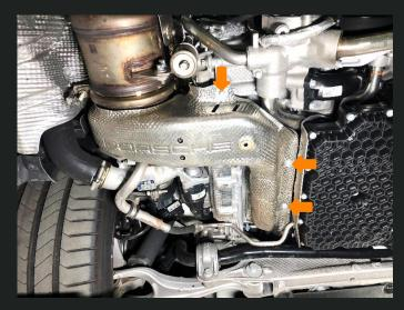
**Step 4**Remove the headers and turbo heat shield.
