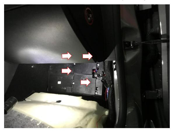
5. Measure the ACC positive power connection control box red power line (positive)
