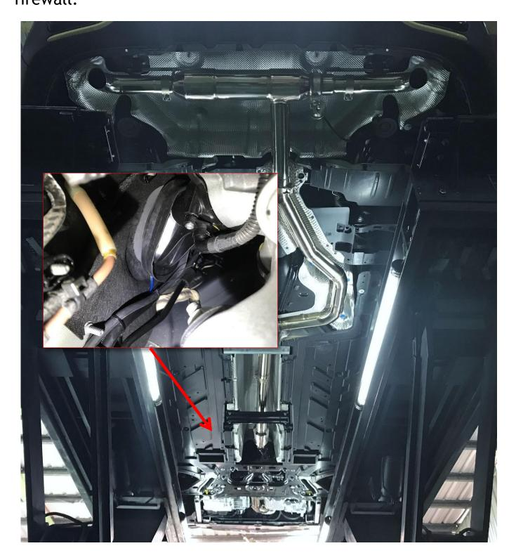
Waring: Pay attention to the steering column to prevent damage to the wires.
