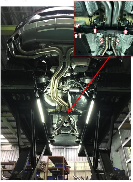
5. The original electronic motor is mounted on the iPE muffler, and the muffler lifting lug and sliding sleeve are replaced.
