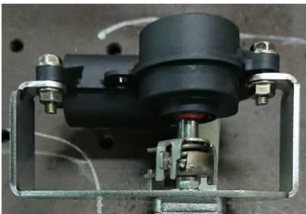
(e) iPE electronic valve motor installation completed (open position).
