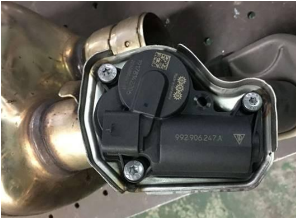
(c) The electronic valve motor is installed on the iPE valve seat and inserted into the OPEN position
