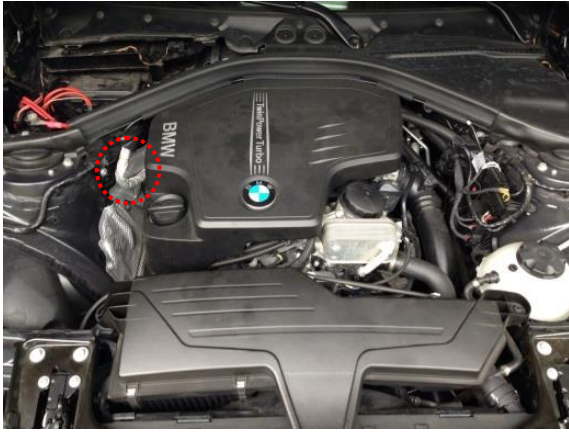
Open the engine hood; the red circle shows the vacuum source.
