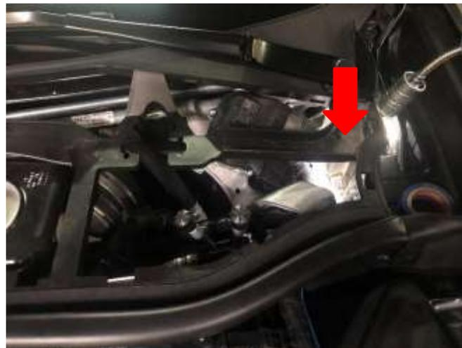
5. Find the fuse box from the left side of brake pedal and measure ACC positive as shown below, and connect the OBD II control box.
