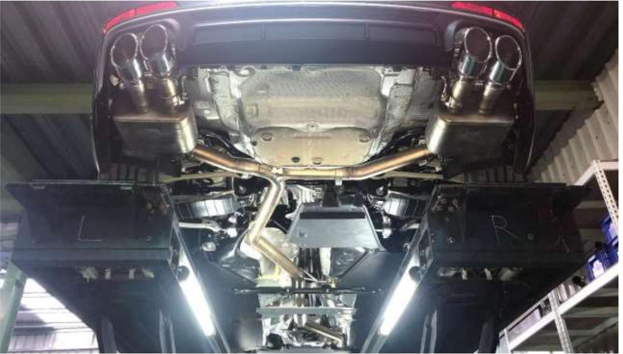
4. Reassemble undercover and support brace. leave at least 15mm between the exhaust and the undercover and support brace.
