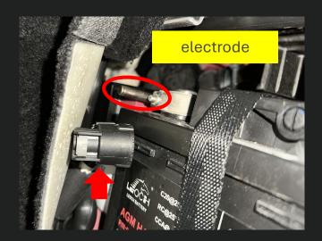
Press and hold to disconnect the high voltage power.
