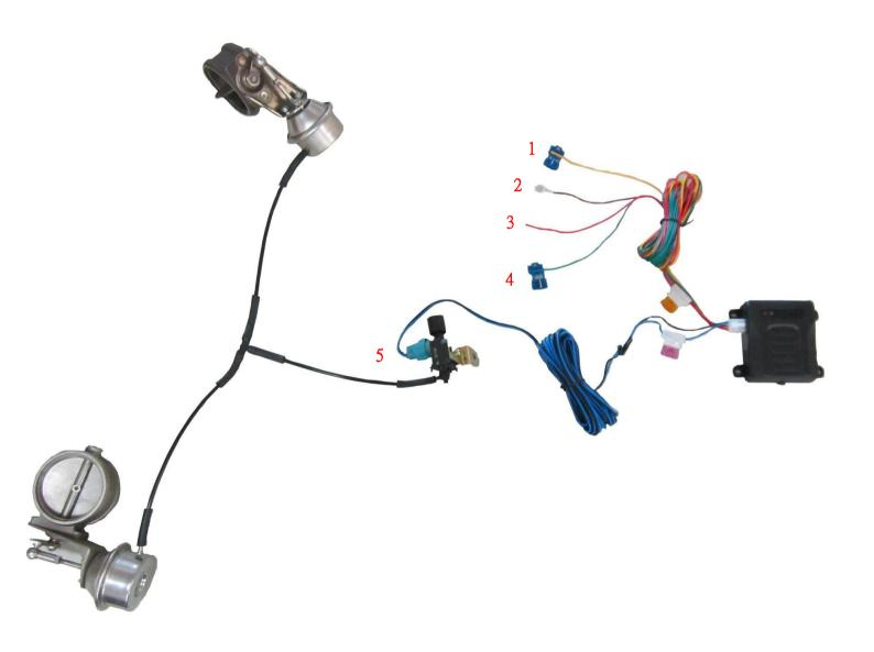
2  $^{\circ}$  YOU CA FIND ELECTRONIC ACCELERATOR IN THE BACK OF GAS PEDAL, THEN PUT TPS(YELLOW CABLE) AND OEM RED CABLE OF ELECTRONIC ACCELERATOR SIDE BY SIDE.
